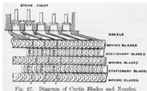
Fig. 27. Diagram of Curtis Blades and Nozzles.
