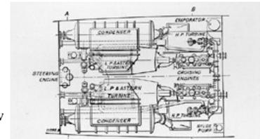
Fig. 41. First set of Combination Machinery—in H.M.S. "Velox."
