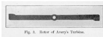
Fig. 3. Rotor of Avery's Turbine.
