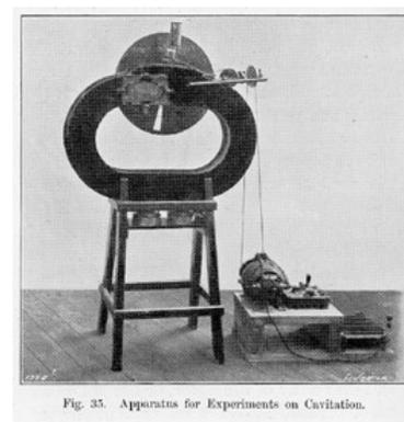
the water asunder, but if the pressure of the atmosphere is removed by an air pump, a model screw will cavitate at a comparatively moderate speed.
